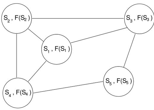
Figure 1: Example of undirected graph representing a search landscape. Each node is associated with a solution  $s_i$  and its corresponding fitness value  $F(s_i)$ . Arcs represent transitions between states by means of  $\varphi$ . Undirected arcs correspond to symmetric neighborhood structures.
