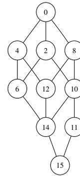
Figure 3: Search graph corresponding to an instance of size 5, with the following symmetries:  $(1\ 2)$ ,  $(1\ 4)$  and a phase shift involving variable  $x_5$ . The maximum node degree is 4 and the minimum is 2.
