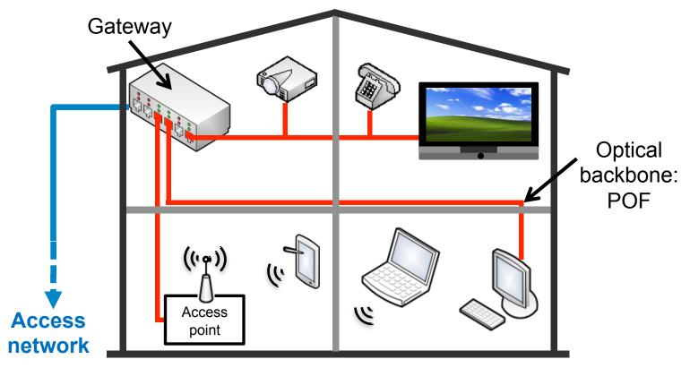
Plastic optical fiber is a promising solution and alternative to copper cables to deliver gigabit and multi-gigabit connectivity within the home or the small office.
